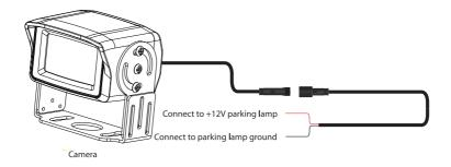
Be sure to test the suspected wires with a digital multimeter as trailer wiring is not universal.
