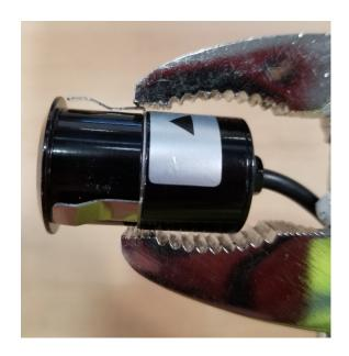
Using a set of Channel Locks or Pliers, position the tool on the clip as shown above and squeeze to compress the clip. Repeat this for all three clips located on the PCAM-220 camera.
