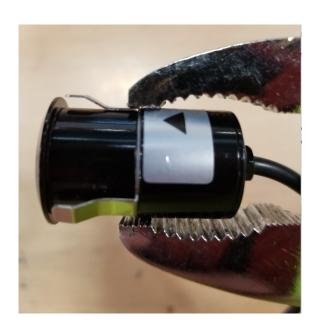
Once completed the clips should be flush with the PCAM-220 body. This will allow the camera to slide into the mounting hole of the JP-MOUNT.
